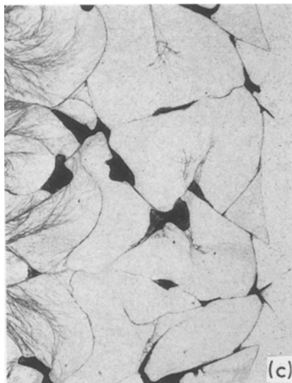
Figure 10 Metallographic section views for a series of impulsively consolidated, monosize 304 stainless steel tubes. (a) 1.1 mm diameter tubes, (b) 1.5 mm diameter tubes, (c) 1.8 mm diameter tubes.
